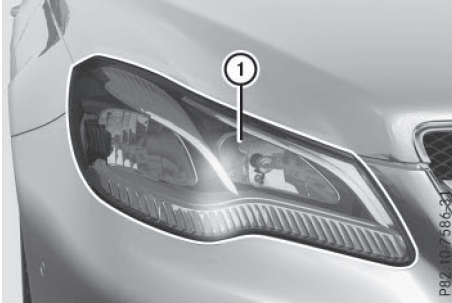
① High-beam headlamp: H7 55 W
