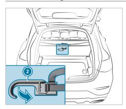
Fold out hook ② on the underside of the cargo compartment floor.
