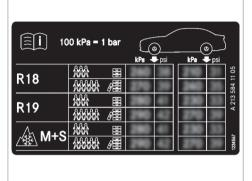
Some tire pressure tables only show the rim diameter instead of the complete tire size, e.g. **R18**. The rim diameter is part of the tire size and can be found on the tire side wall ( $\rightarrow$  page 474). Be sure to also observe the following further related subjects:
