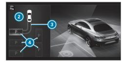
The media display shows the view of Active Parking Assist. Area ② displays detected parking spaces ③ and vehicle path ③.
