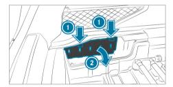
Push retaining clamps (1) on the cover downwards to release them and fold out the cover in the direction of arrow (2).
