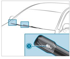
Remove protective film (1) from the maintenance display on the tip of the newly installed wiper blades.
