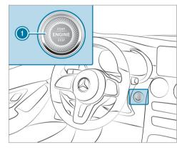
To switch on the power supply: press button (1) once.
