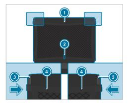
Open cargo compartment floor 1,  $(\rightarrow page 119)$  swing it upwards to an angle
