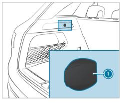
Lift up cap ① of the socket and insert the plug of the device.
