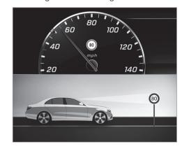
If a change in the speed limit is detected and automatic adoption of speed limits is activated. the new speed is automatically adopted as the stored speed ( $\rightarrow$  page 241).
