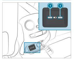
You can charge a USB device, e.g. a mobile phone, at USB ports 1 using a suitable charging cable.
